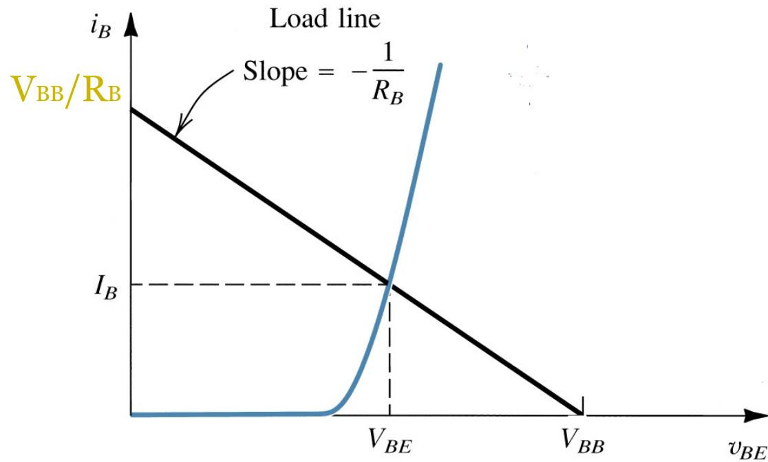
$$I_B = (V_{BB} - V_{BE})/R_B$$
