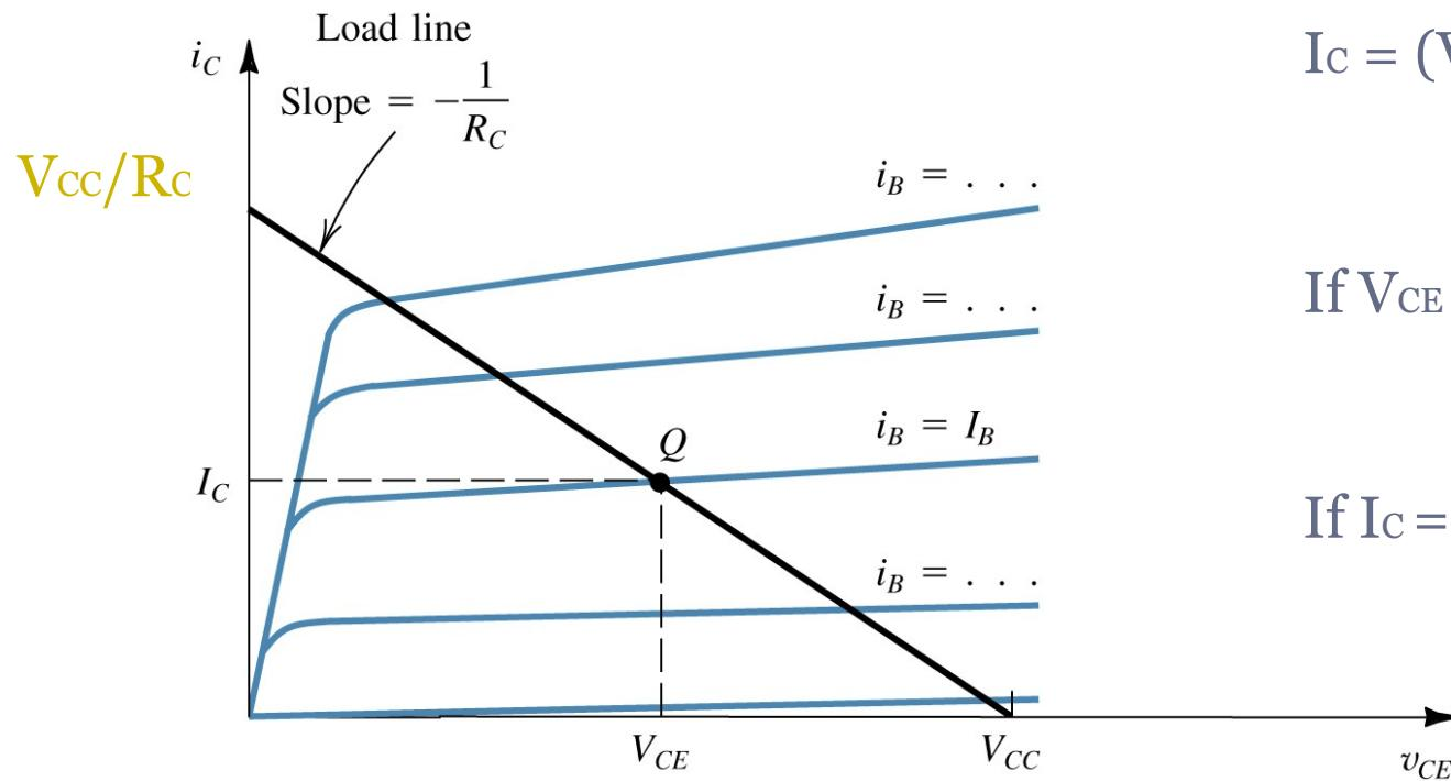
$$I_C = (V_{CC} - V_{CE})/R_C$$
