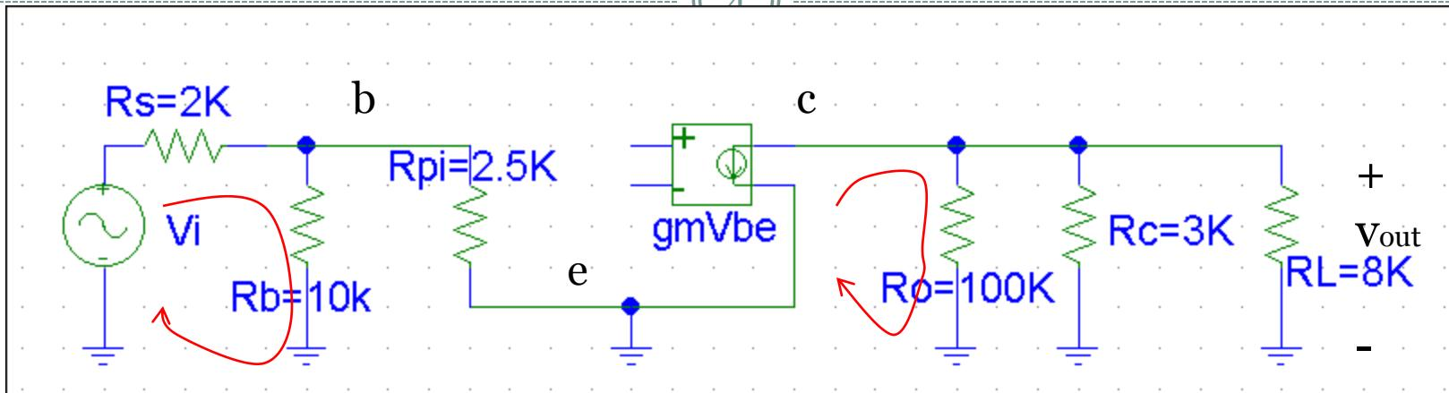
$$V_{be} = (R_b || R_{pi}) / [(R_b || R_{pi}) + R_s] V_i$$
