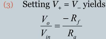
Notice: The closed-loop gain  $V_{\rm o}/V_{\rm in}$  is dependent upon the ratio of two resistors, and is independent of the open-loop gain. This is caused by the use of feedback output voltage to subtract from the input voltage.
