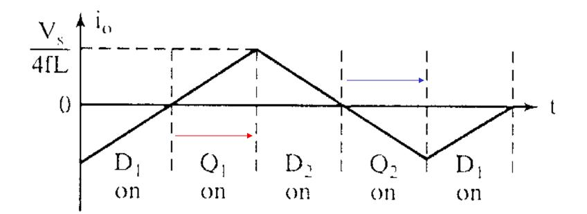
Transistors are only switched on for a quarter-cycle, or  $90^{\circ}$
