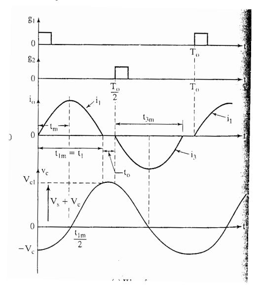
To avoid a short-circuit across the main dc supply,  $T_1$  must be turned OFF before  $T_2$  is turned ON, resulting in a "dead zone".
